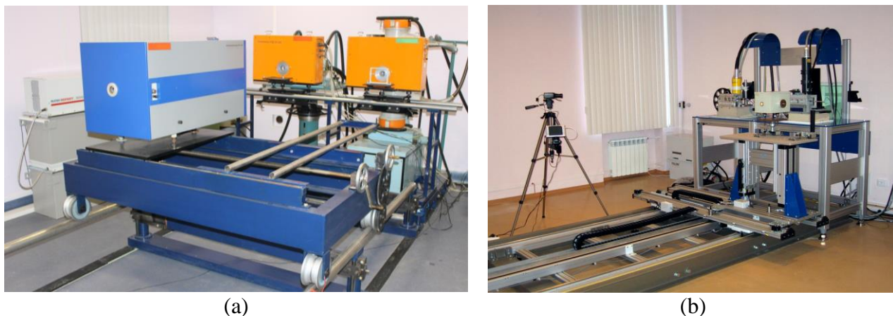
Figure 1. The primary standard facilities for x-rays air kerma measurement: for medium-energy x-rays (a); for low-energy and mammography x-rays (b)
