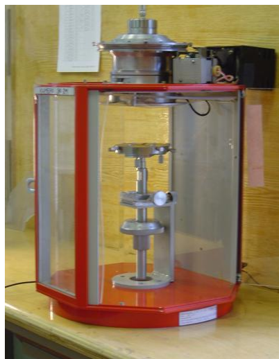
Figure 2. Primary standard extrapolation chamber for beta radiation absorbed dose in tissue measurement
