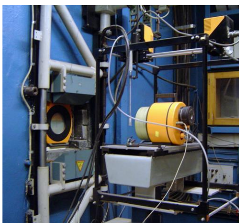
Figure 3. Primary standard thick-walled ionization chamber IKV-6 in the field of accelerator BETATRON B 50/50
