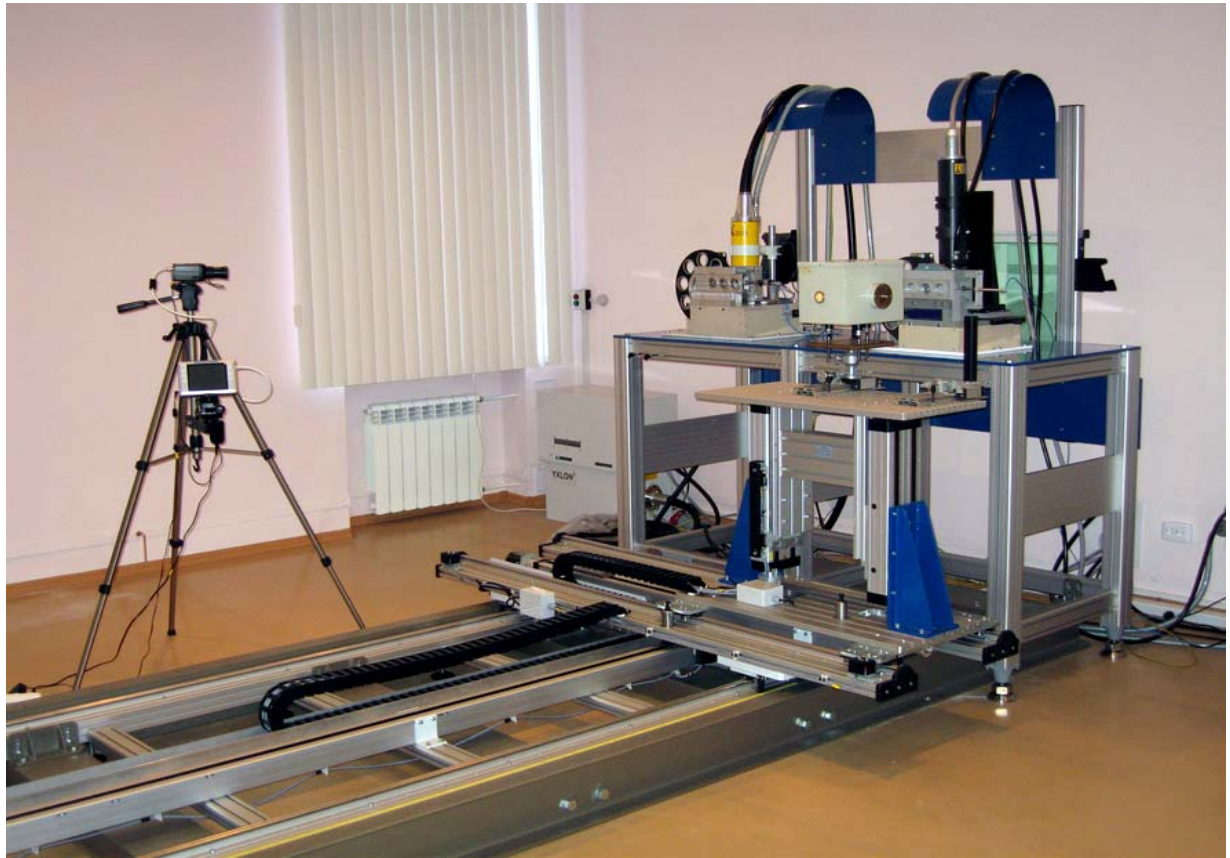
Figure 1. The VNIIM low-energy and mammography X-rays air kerma primary standard facilities
