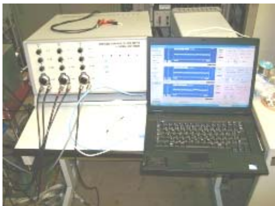
Figure 4 The new compact-size control system for the calorimeter.
