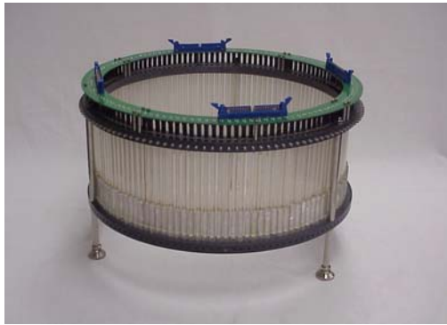
Fig. 5. Left: A 35.5 cm-diameter, 128-element submersible ultrasonic array for tomographic temperature reconstruction. Right: Temperature profile reconstructions in a water phantom from a fan beam tomographic acoustic experiment with 64 projections, 45 rays per projection with a 30 s exposure from a heat lamp as a radiation source. Area dimensions: 300 pixels = 230(mm); Relative height of the temperature dome is about 8
