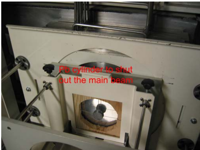
Figure 5 Photograph of the stopper setting
