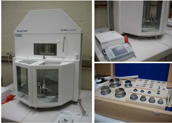
New mass comparator and its ancillary class E1 weight set
