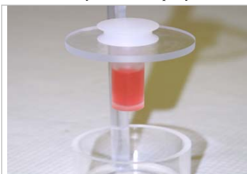
Epoxy-based ^{68}\text{Ge} “mock” syringe artifact standard developed by RadQual, LLC for the calibration of dose calibrators for ^{18}\text{F} . The epoxy is colored in this photograph only for visual detail.
