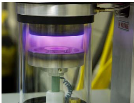
Coating a thin-film source with gold for an anticoincidence measurement.
