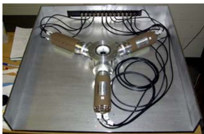
NIST TDCR system, open view showing the photomultiplier tubes (PMT's) Robotic sample changer-system for ionization chamber
