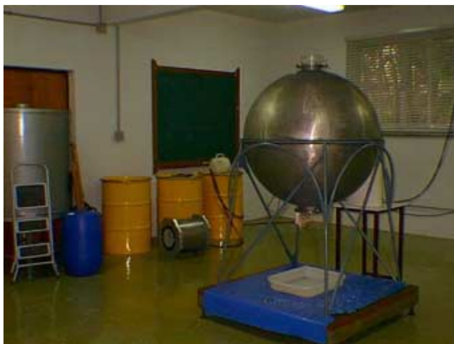
Figure 1. Manganese Sulfate Bath located at LNMRI/LN – Laboratório de Nêutrons
