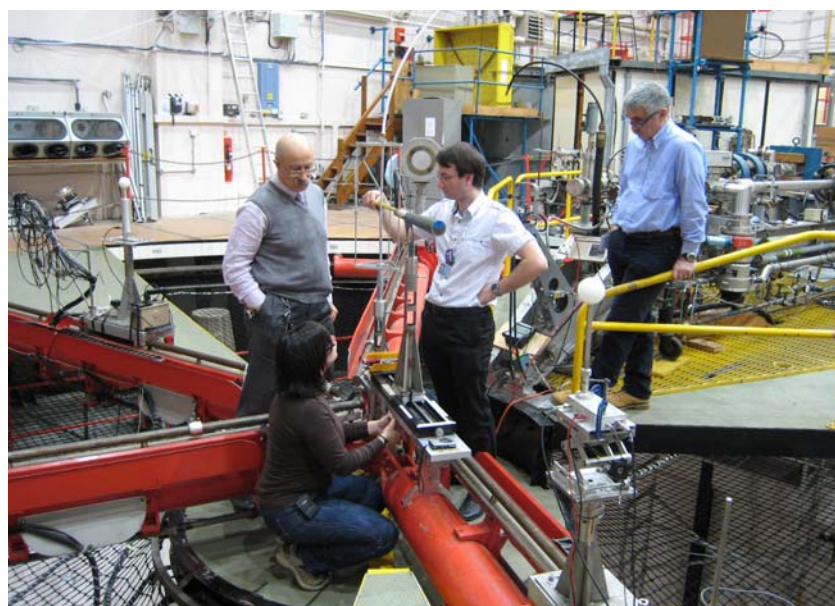
Figure 10. Setting up the UAB and INFN Bonner spheres in the low scatter facility at NPL
