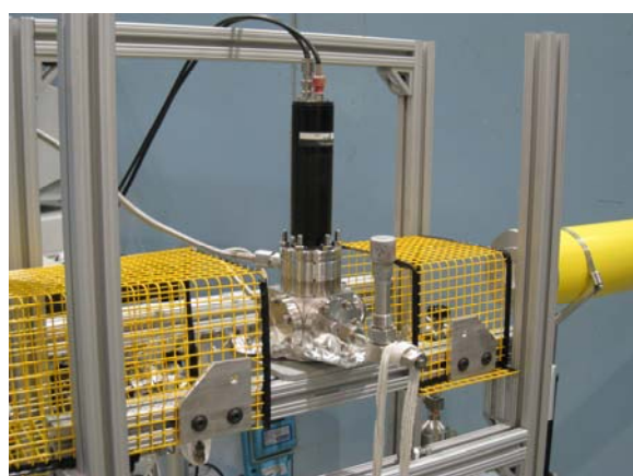
The 'LND' detector taking data at NG6-A beam-line in the guide hall
