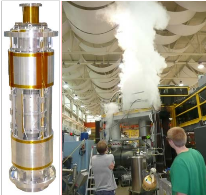
(Left) Ioffe type magnetic trap (Right) Successful test quench of the full magnetic trap in its final horizontal position.
