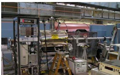
Figure 1: Photon detection is done by twelve BGO crystals viewed by avalanche photodiodes forming an annular ring around the neutron beam.
