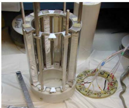
Figure 1: Photon detection is done by twelve BGO crystals viewed by avalanche photodiodes forming an annular ring around the neutron beam.
