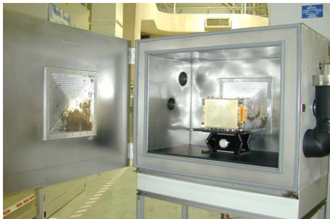
Sample chamber with 100 cm 2 cell inside. Windows on front and back are for neutron transmission.
