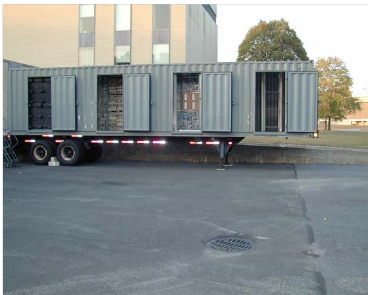
A cargo container test bed with three massive cargo regions as needed for testing under ANSI N42.41 is being set up for use at NIST in Gaithersburg or at other sites
