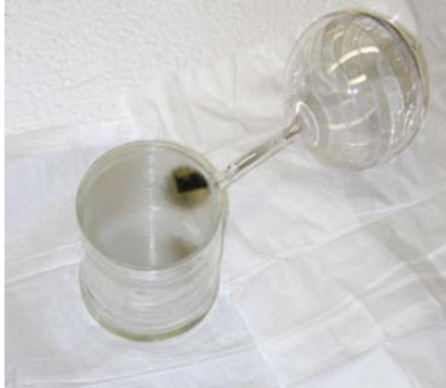
"Double cell" for continuous optical pumping in high flux beams. The spherical volume is maintained at \sim 200\text{ C} and illuminated with laser light for optical pumping, and only the flat-windowed, spin filter cell is in the neutron beam
