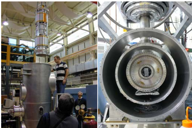
(Left) Lowering the new magnetic trap into the cryostat. (Right) After installation the end view of the magnet helium bath and heat shields on the NG6-u beamline. The thermally isolated ultra-pure helium cell (with test weight) is seen suspended from three Zylon
