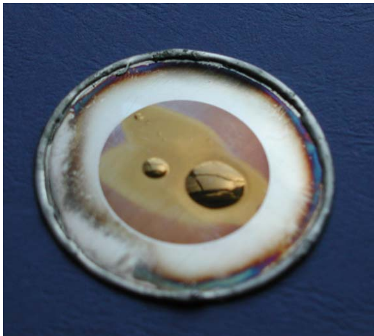
Figure 2. Tungsten-backed scandium target exhibiting typical blistering after proton bombardment
