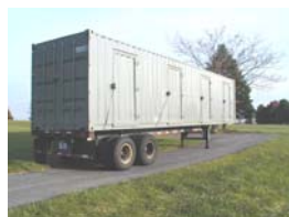
A cargo container test bed with three massive cargo regions as needed for testing under ANSI N42.41 is being set up for use at NIST in Gaithersburg or at other sites
