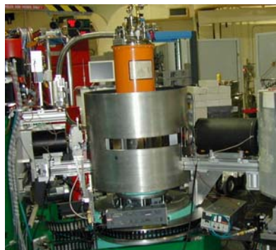
The BT7 thermal triple-axis spectrometer with {}^3\text{He} spin filters to polarize and analyze the neutron beam. After exiting the monochromator drum (green structure on the left), the neutron beam passes through the polarizer solenoid (small black cylinder) to the sample; the scattered beam passes through the analyzer solenoid (larger black cylinder) to the detector (aluminum cylinder on the right).
