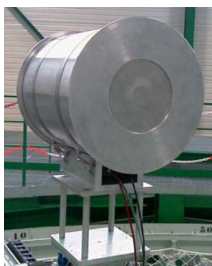
Figure 2 : IRSN long counter on its support, manufactured on basis of the geometry defined by Monte-Carlo study
