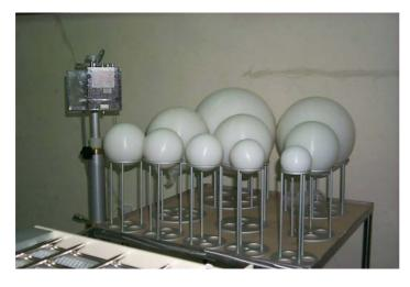
12" diameter and originally designed PTB, by Braunschweig. The response matrix is calculated by the small modification of original PTB BS's response matrix, considering the difference of the density and the size of the spheres. The normalization of the response matrix is determined by the measurement
