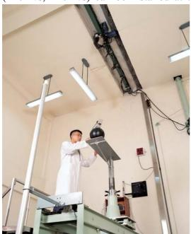
$(^{252}Cf$  with the neutron emission rate of  $\sim 10^8$  n/s) can be controlled remotely. The moving arms for the calibration and test of the neutron detector can be moved about 2 m (the minimum distance from the source is  $\sim 20$  cm).
