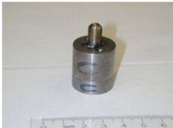
Figure. Neutron Sources for Homeland Security. Californium-252 sources spontaneously emit fission neutrons. These sources were embedded in a 1-cm thick steel shell. This has the effect of suppressing gamma rays and providing a rugged container for field use.
