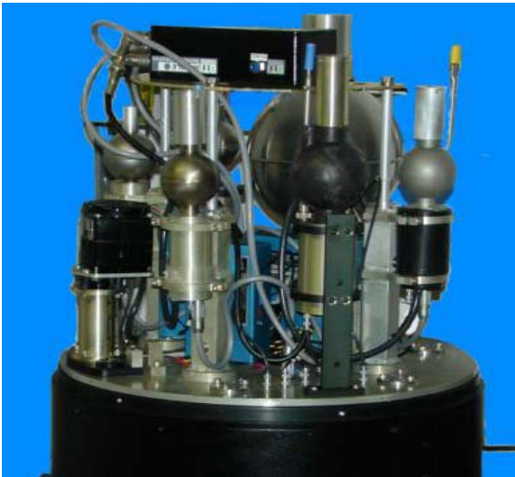
Figure: Rotating Spectrometer (ROSPEC). ROSPEC combines several neutron detectors into a single system to measure the neutron spectrum from thermal neutron energy to 18 MeV. The detectors rotate so that all detector sample the same volume.
