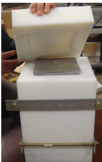
Fig.4. Simple emission rate detector composed of a polyethylene moderator and two ^3\text{He} proportional counters
