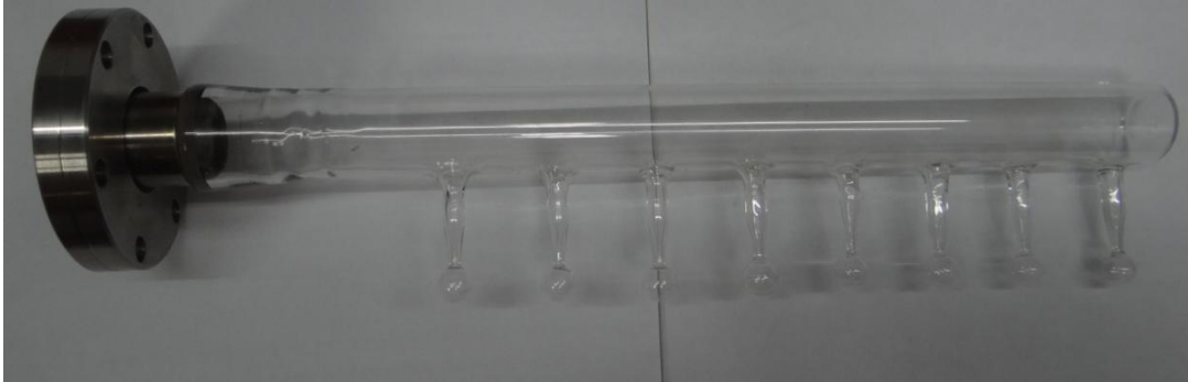
Fig. 14: Glass Manifold consisting of bulbs
