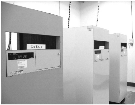
Figure 3. The cesium clocks in the clock room located on a basement floor.
