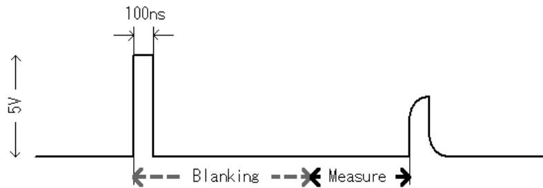
Figure 7. Explanation of the cable delay measurement. A pulse wave is injected to a cable. We measure the time interval between an injected pulse and reflected pulse. To exclude the noise such as a reflection from impedance unbalance in halfway, the blanking function of a time interval counter is effective.
