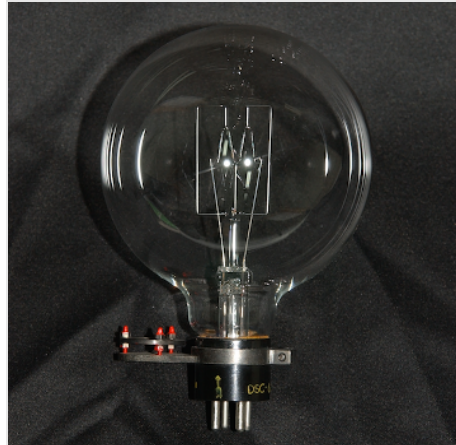
Fig. A6.1 Coil-M-type luminous intensity standard lamp (55 V-330 W)
