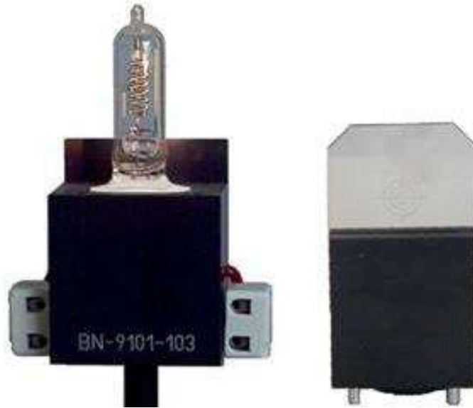
Figure 4.1. Measurement artifact – tungsten halogen lamp of FEL 120V-1000W type mounted by Gigahertz-Optik with alignment jig (right).
