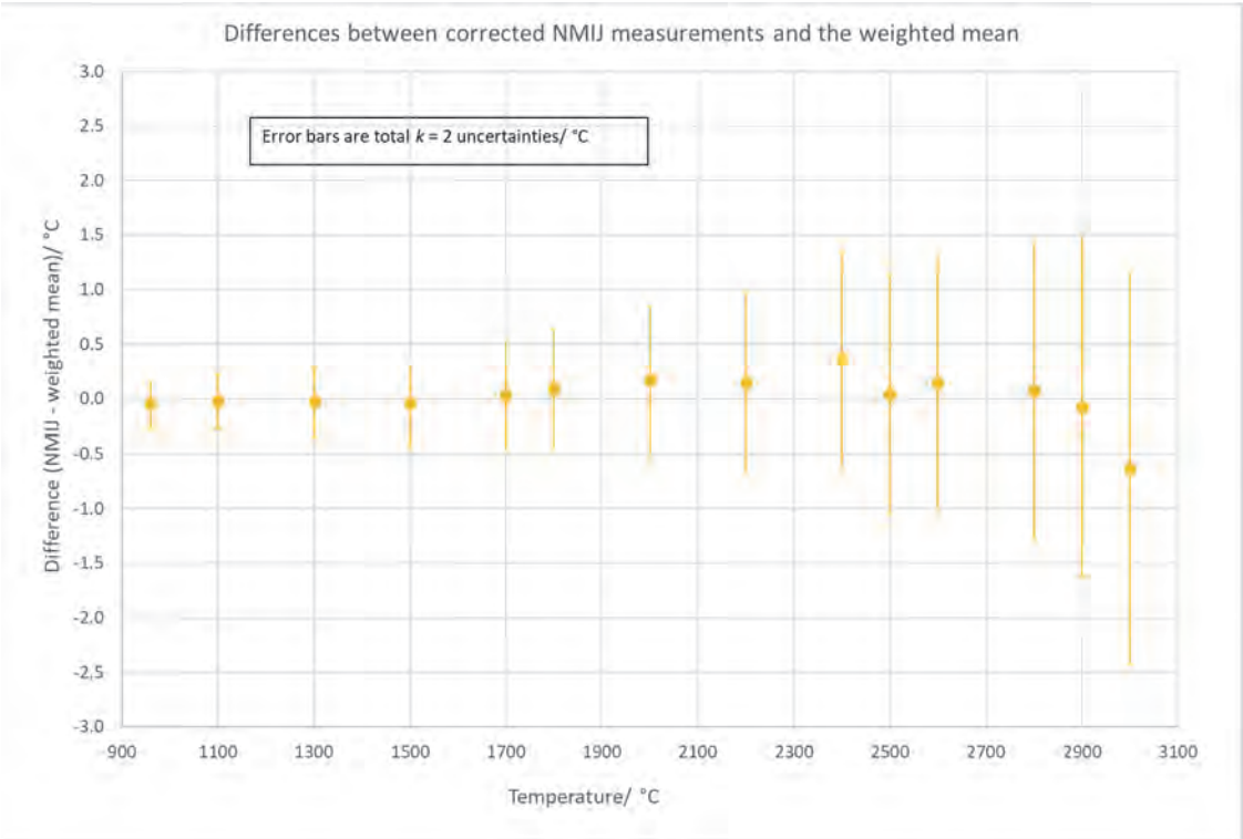
Figure 133 - difference between the NMIJ results and the weighted mean ( k = 2 total uncertainties)
