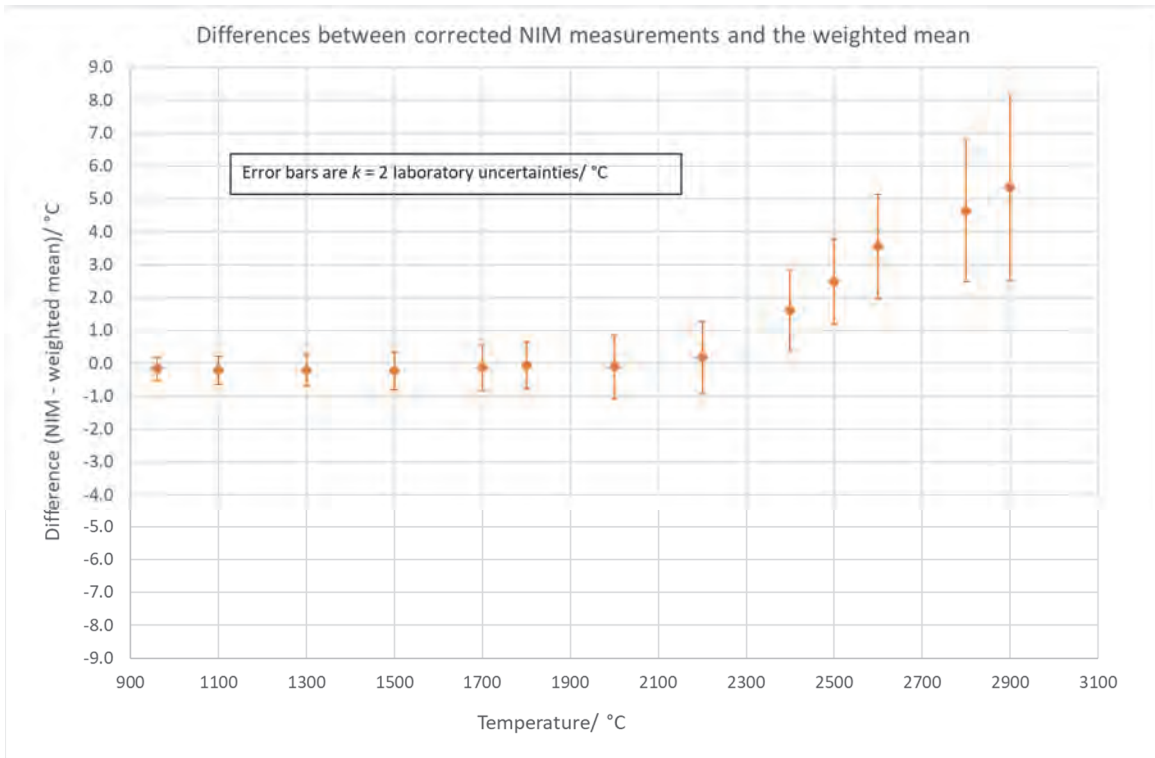
Figure 134 - difference between the NIM results and the weighted mean ( k = 2 laboratory uncertainties)
