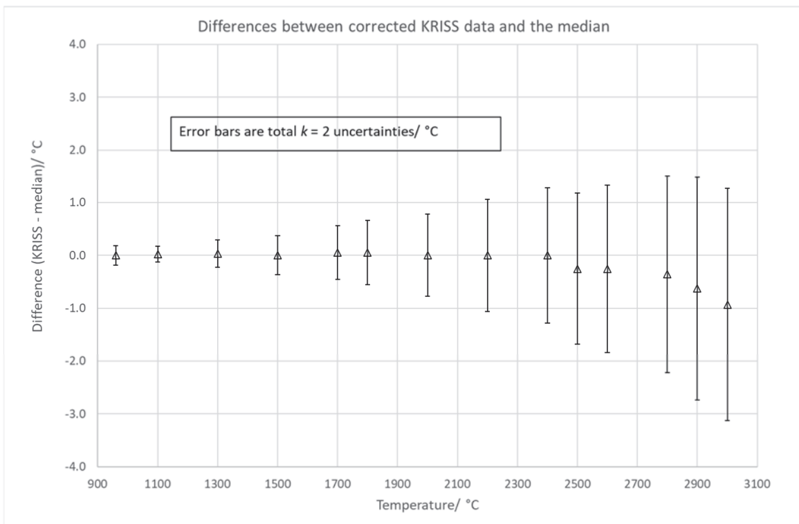
Figure 43 – difference between the KRISS results with the LP3 and the median ( k = 2 total uncertainties)
