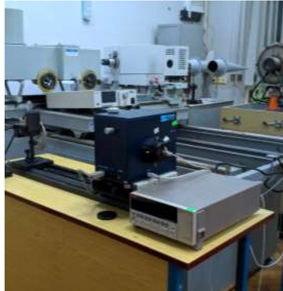
Figure 5.3.2. Facility for measuring relative spectral irradiance of FEL lamps
