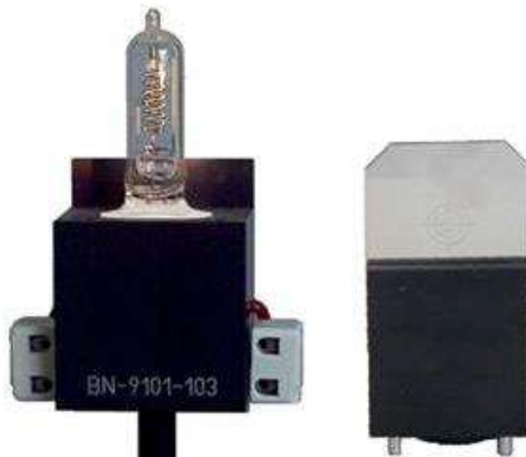
Figure 4.1. Measurement artifact used by all participants except NSC IM – tungsten halogen lamp of FEL 120V-1000W type mounted by Gigahertz-Optik with alignment jig (right).
