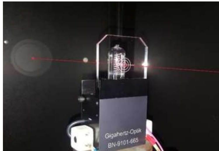
Figure 4.3. Aligning the lamp.
