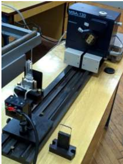
Figure 5.3.2. Facility for measuring relative spectral irradiance of FEL lamps
