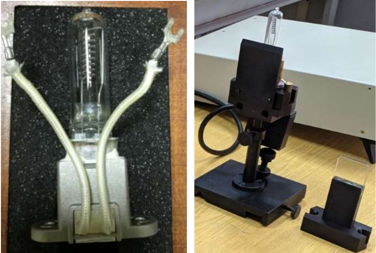
Figure 4.2. Measurement artifact used by NSC IM – tungsten halogen lamp of FEL 120V-1000W type mounted by Newport: in a traveling box (left), with holder and alignment jig (right).
