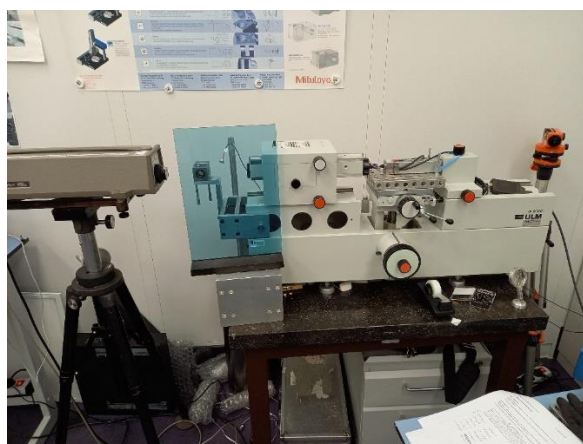
Figure 2. Calibrating the transducer in the horizontal position on the ULM with a laser interferometer.
