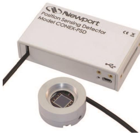
Figure 3: Position sensing detector for adjusting the laser beam to the measurement direction
