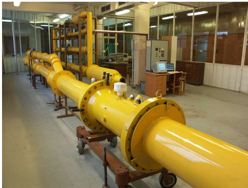
Figure 9 – Test bench in LEI with reference meters
