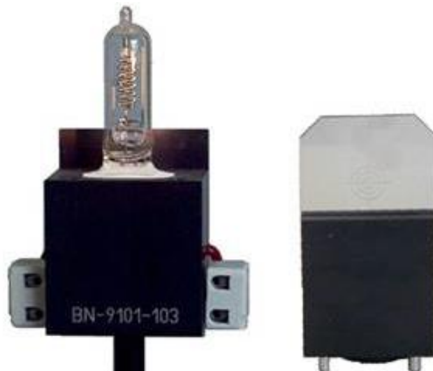
Fig.1. Measurement artifact – tungsten halogen lamp of FEL 120V-1000W type mounted by Gigahertz-Optik with alignment jig (right).
