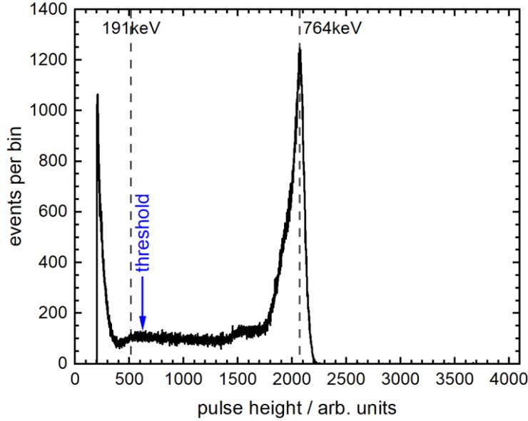
**Fig. 2** Pulse height distribution of a low-pressure  $^3\text{He}$  counter
