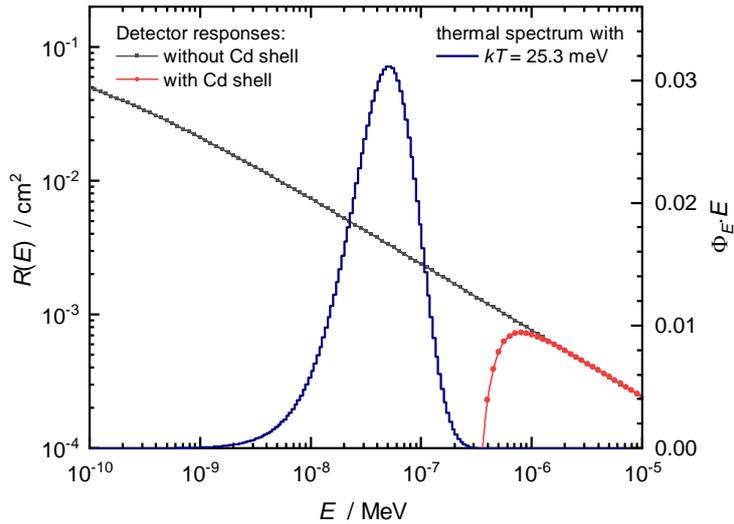
**Fig. D1** Response function of SP9 counter (left axis). The response of the SP9 counter was calculated using the MCNP for parallel neutron beam perpendicular to the symmetry axis of the counter. Also shown is the relative Maxwellian spectral fluence distribution for  $kT = 25.3 \text{ meV}$  (right axis).
