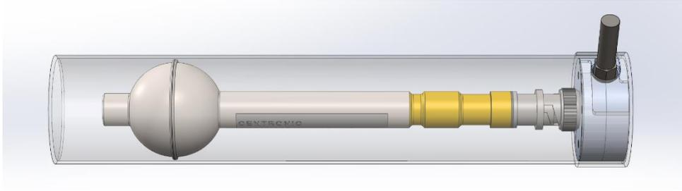
**Fig. C3** Schematic diagram of the bare SP9 counter in cadmium shell.
