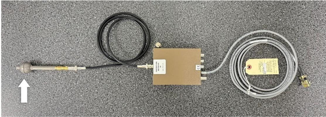
**Fig. C5** Measurement system connection diagram (up panel) and the connection status of the detector, high-voltage signal cable and the pre-amplifier (down panel)
