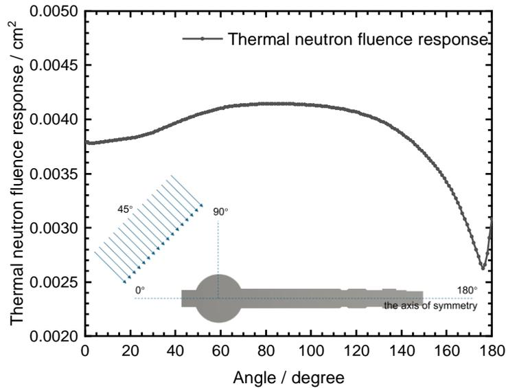
**Fig. E1** Directional dependence of SP9 counter response. The response of the SP9 counter was calculated using MCNP for parallel neutron beams with a Maxwellian distribution for the temperature parameter  $KT$  of 293.6 K. 0°, the angle between the neutron beam and the detector symmetry axis, represents that the beam is incident parallel to the symmetry axis from the direction of the counter “nose”, and 90° represents that it is incident perpendicular to the symmetry axis.
