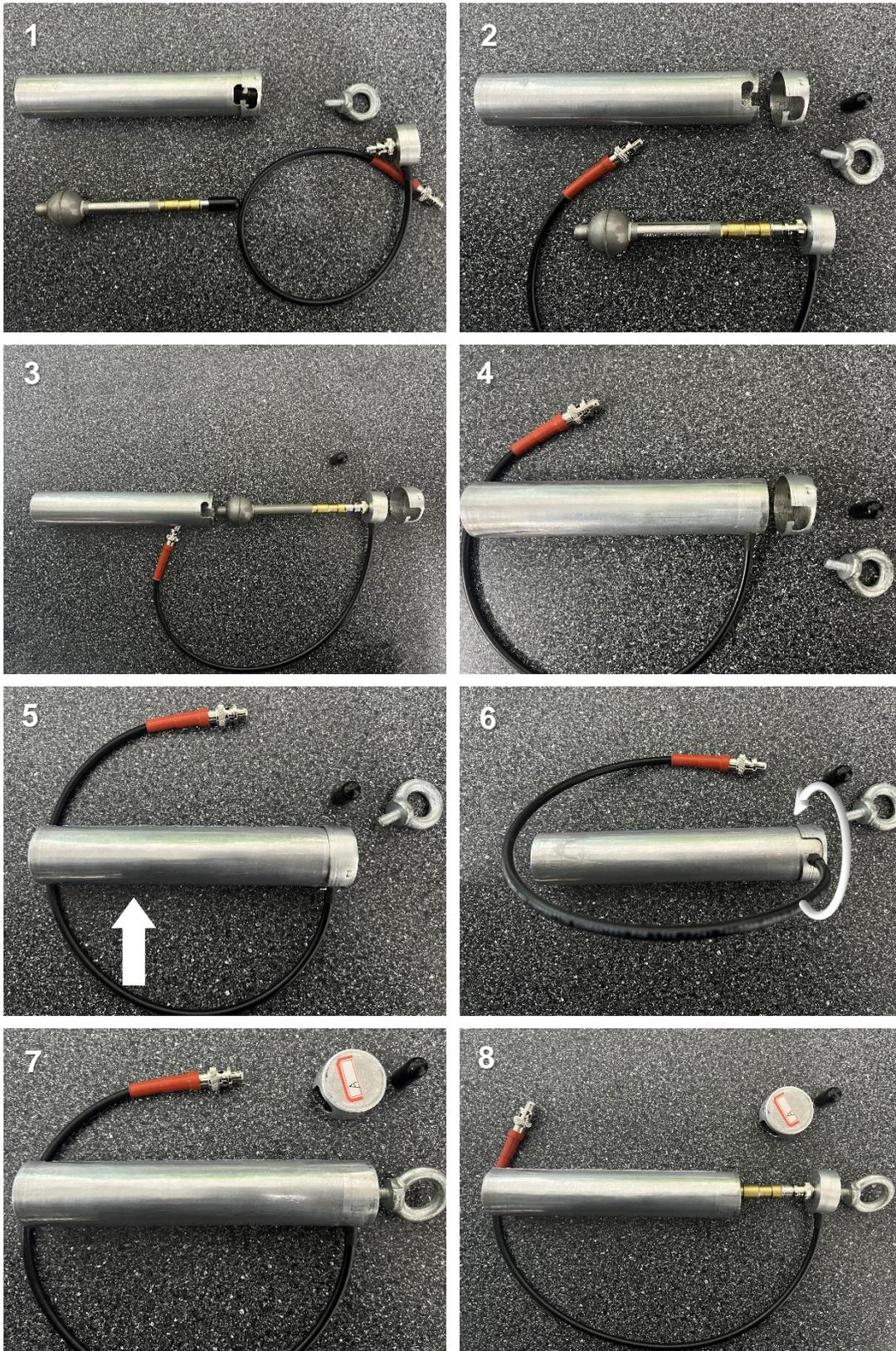
**Fig. C2** Insertion of the bare counter into the cadmium shell.
