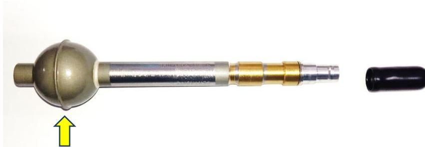
**Fig. C1** SP9 counter and the irradiation direction
