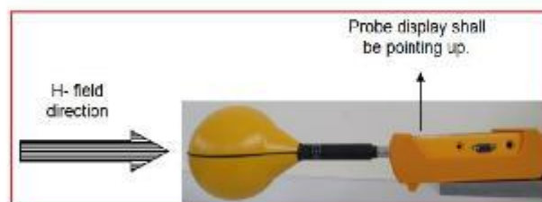
Figure 2. The position of magnetic field probe during comparison measurements
