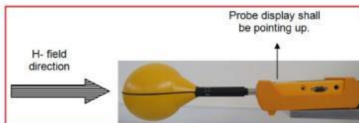
Figure 2: Position of ELT-400 during measurements
