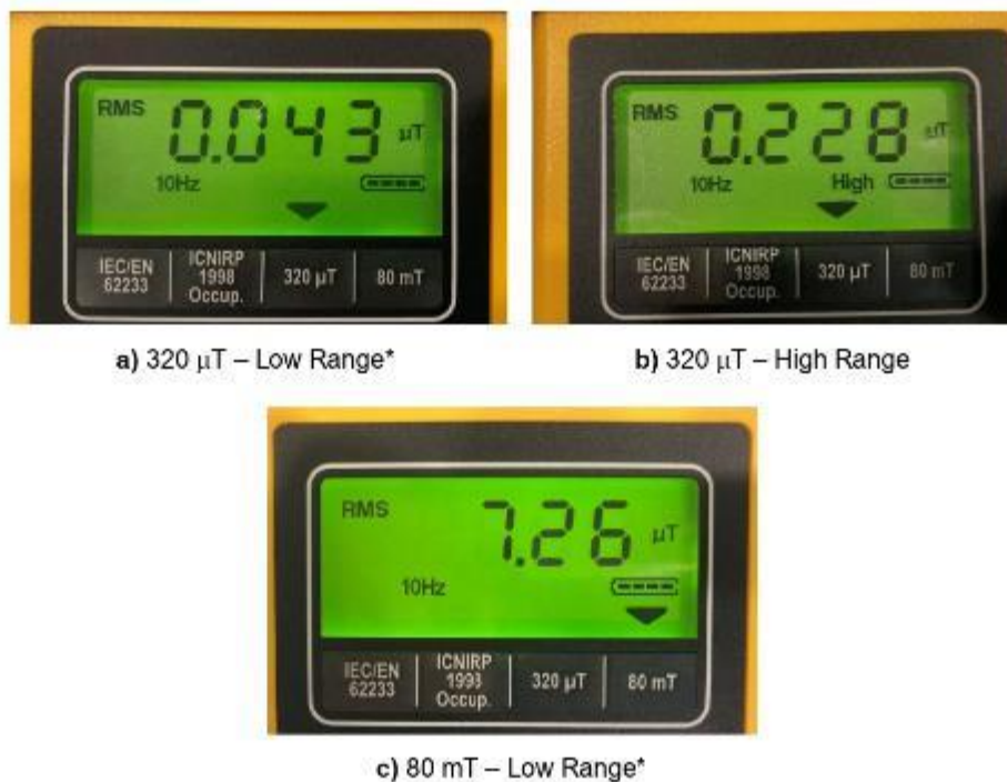
Figure 3. Measurement settings of the ELT-400 during measurements
