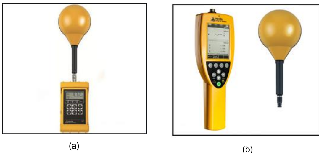
Figure 1. The photo of the travelling standards, a) ELT 400, b) HF3061 with NBM-550
