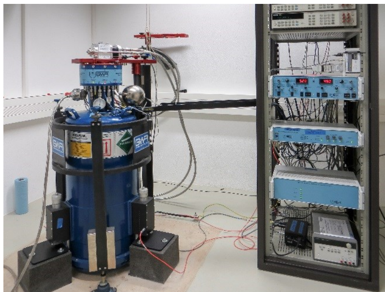
Figure 2. GWR SG030 of BKG is registering temporal gravity variations at pillar WET_GA continuously since 2010
