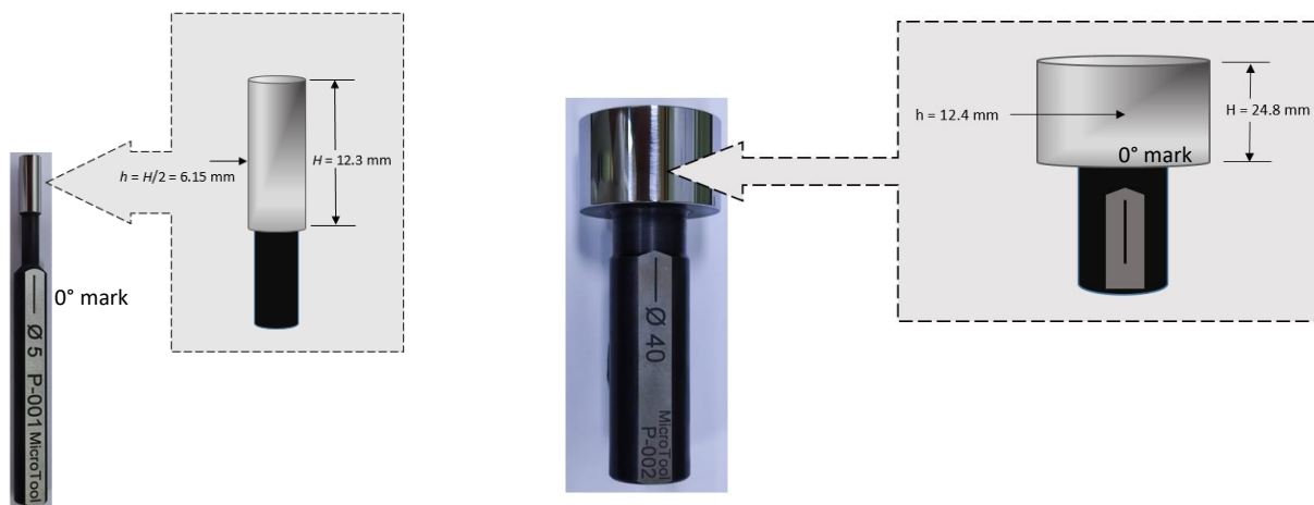
Figure 4. Measuring direction on the plugs: 5 mm plug (left) and 40 mm plug (right)
